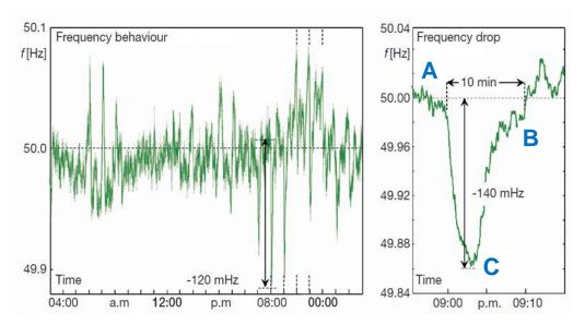
Figure 3: Current operational frequency behaviour in Continental Europe (Source: University of Stuttgart)
