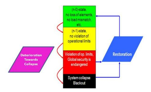
Figure 7: System States in the framework of the OS NC (Source: ENTSO-E)
