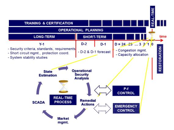
Figure 23: Structural interfaces and dependencies in System Operation (Source: ENTSO-E)
