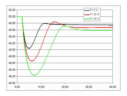
Figure 4: Impact of PV penetration on island networks in case of loss of generation (Source: EDF)
