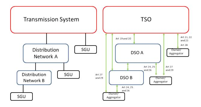
Figure 9: Comparison of the electric connection and the flow of information (Source: ENTSO-E)
