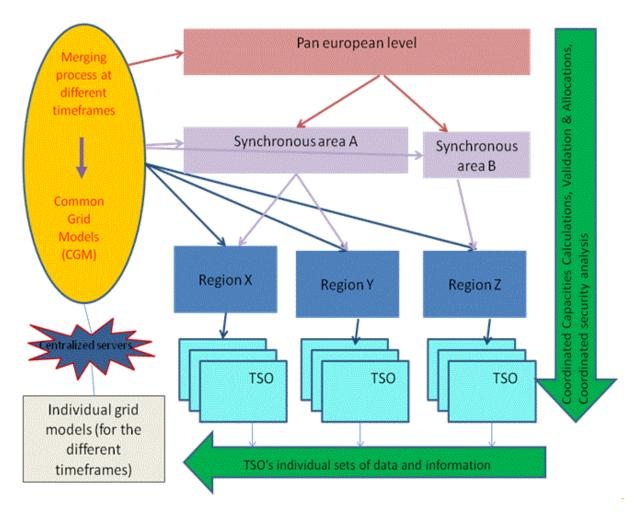
Figure 12: Overview of CGM building process: data and information exchange (Source: ENTSO-E)
